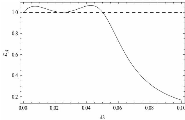
**Fig. 4.** Optimized amplitude dynamic error
